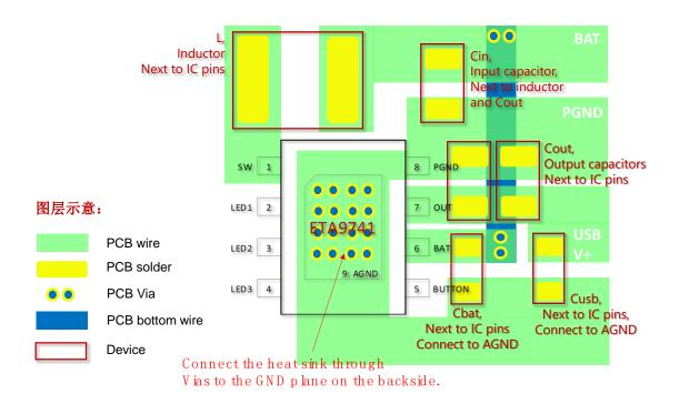
Please have  $C_{IN}$ ,  $C_{OUT}$ , and L placed just next to the IC pins so that the power traces are kept to the shortest to achieve a good performance of ETA9741 and good EMI.
