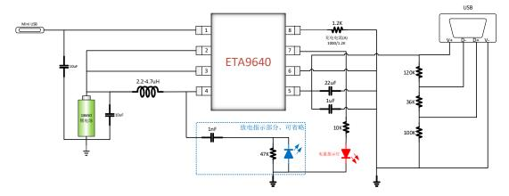
The ETA9640 is designed dedicated for a Li-ion powered system with 1A USB output port, such as portable power bank. A complete application circuit is shown above, where one can find very few peripheral devices needed. The 120K/36K/120K serial resistor is just for the iPhone charging port setup, which is not necessary for all systems. One can also simply short the D+ and D- pin of the USB output port to achieve the same function.
