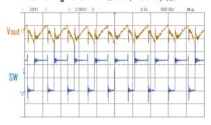
Transient Response Waveform: V<sub>IN</sub>=3.6V, Vout=5V, I<sub>OUT</sub>= 0.1-1A
