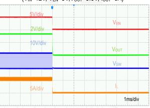
Startup from VIN (V<sub>IN</sub>=12V, V<sub>OUT</sub>=3.3V, I<sub>OUT</sub>=6A)
