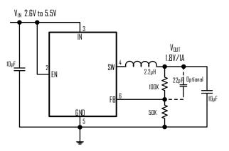
1.8V/1A 1.5MHz Step-Down Converter
