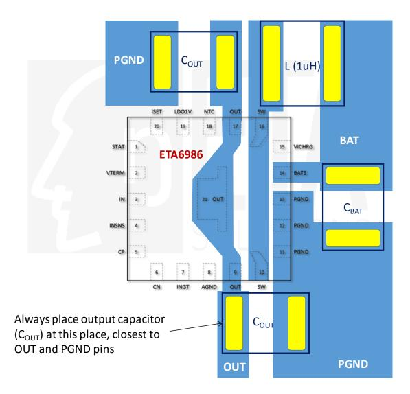
Please try to place the Cout, L, and Cbat as suggested by the illustration above. The Cout has to be placed just next to the chip with shortest wire to the OUT and PGND pins. And SW wire goes underneath the chip and connected by a power inductor just next to the Cout. With the Cin placed beside and the shortest SW trace, a very tight and small power loop is achieved, so as to improve EMI characteristics.
