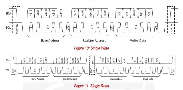
Device address is understood value of A[7:0] while A[0] is "0". This is also the address to write the data to the device registers. To read data from register, sending the command to address with A[0] is "1". Register address are in RA[7:0]. Data to or from register are D[7:0].
