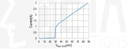
Figure 3: BATFET Current at Entering Supplement Mode
