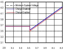
Figure 2: System Voltage vs Battery Voltage
