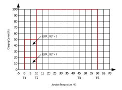
Figure 5: JEITA Profile: Charging Current
