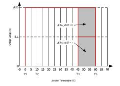
Figure 6: JEITA Profile: Charging Voltage
