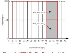
Figure 6: JEITA Profile: Charging Voltage
