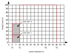
Figure 5: JEITA Profile: Charging Current
