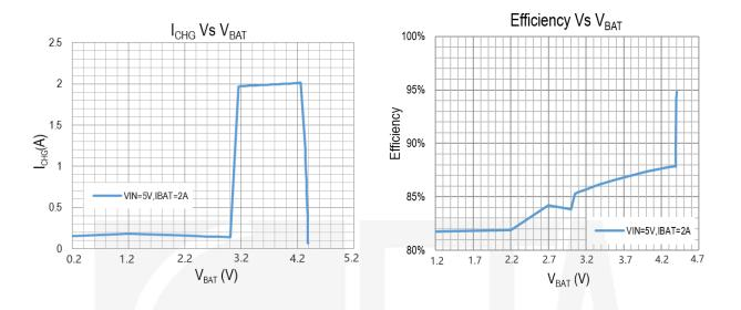
Complete charging cycle of a 10000mAH battery at 2A charge current -
