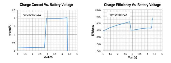
Complete charging cycle of a 5600mAH battery at 2.15A charge current
