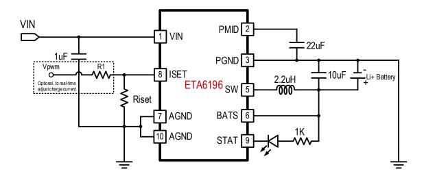
As given by above application circuit, one can real-time adjust the charge current by a PWM signal with different dutycycle. The Vpwm is the RC filtered voltage of the PWM signal, and it will change linearly with the duty-cycle of the PWM signal. Followings are 2 examples of charge current's relationship to Vpwm. Please contact ETA engineers if one wants to have specific real-time charge current setting, the choosing of R1 and Rset value will be provided quickly.
