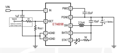
As given by above application circuit, one can real-time adjust the charge current by a PWM signal with different dutycycle. The Vpwm is the RC filtered voltage of the PWM signal, and it will change linearly with the duty-cycle of the PWM signal. Followings are 2 examples of charge current's relationship to  $V_{PWM}$ . Please contact ETA engineers if one wants to have specific real-time charge current setting, the choosing of R1 and Rset value will be provided quickly.
