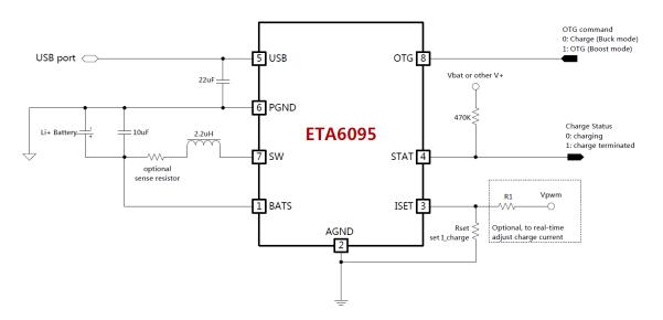
As given by above application circuit, one can real-time adjust the charge current by a PWM signal with different duty-cycle. The Vpwm is the RC filtered voltage of the PWM signal, and it will change linearly with the duty-cycle of the PWM signal. Followings are 2 examples of charge current's relationship to Vpwm. Please contact ETA engineers if one wants to have specific real-time charge current setting, the choosing of RI and Rset value will be provided quickly.
