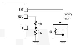
Where  $R_{NTC\_HOT}$  is the value of the NTC resistor at the upper bound of its operating temperature range, and  $R_{NTC\_COLD}$  is its lower bound. The two resistors,  $R_{TS1}$  and  $R_{TS2}$ , independently determine the upper and lower temperature limits. This flexibility allows the ETA6071 to operate with most NTC resistors for different temperature range requirements. Calculate  $R_{TS1}$  and  $R_{TS2}$  as follows:
