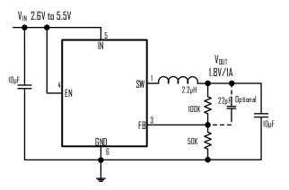
1.8V/1A 1.5MHz Step-Down Converter
