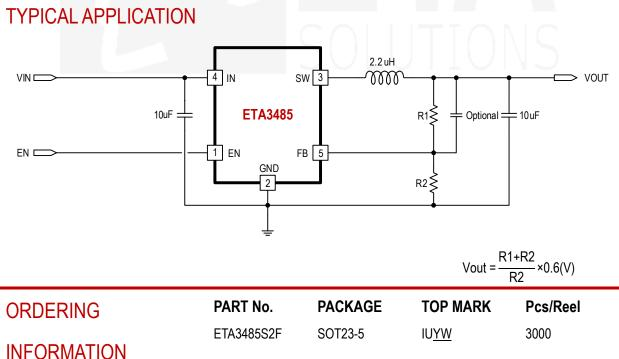
ETA3485 is housed in a tiny SOT23-5L
