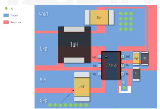
Cin has to be placed very close to VIN and GND pins.
