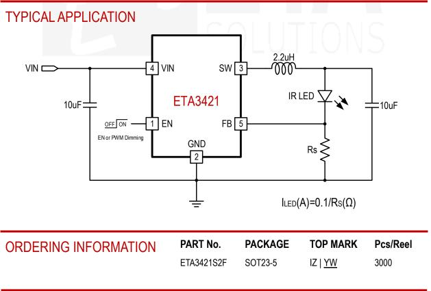
ETA3421 is housed in a tiny SOT23-5 package.
