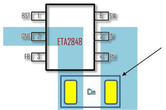
Always keep input capacitor (Cin) as close to the IN and GND pin as possible. Please do wire the GND trace underneath the ETA2848 package body and achieve the shortest way to the IN pin. It is not allowed to connect the capacitor to the GND pin through via!
