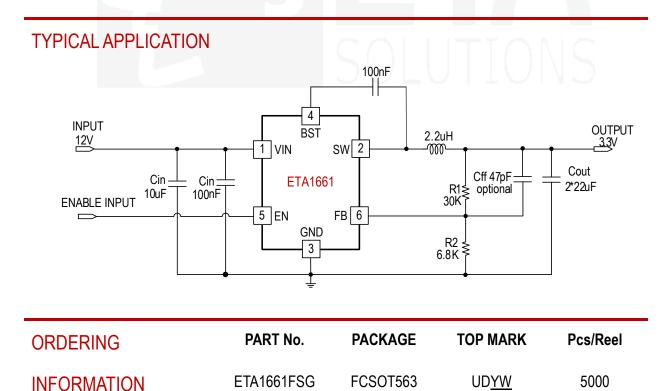
ETA1661 is available in a tiny SOT563 package.
