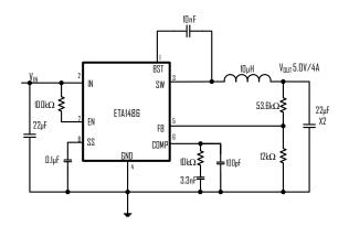
4A Wide Input Step Down Synchronous Converter
