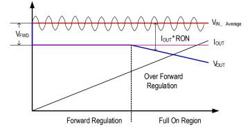
The forward regulation voltage for the ripple remover is 75mV. When the difference between  $V_{OUT}$  and  $V_{IN\_Average}$  is less than 75mV, the ripple remove function will work to filter out the input ripple, so that IC can provide a stable output voltage.
