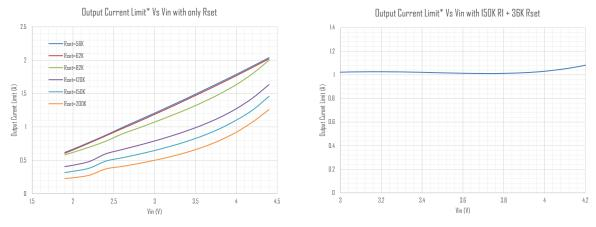
\*Output current limit is the output current measured at Vout=4.75V
